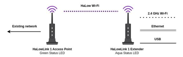
This will require **two** HaLowLink devices, and will make a HaLow link a transparent part of your network, functioning just like an Ethernet cable.
