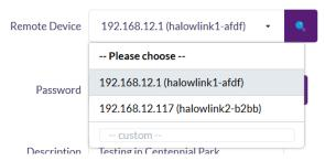
to find a device which is connected to the same network as the local HaLowLink 1, a user may enter any IPv4 address into the 'custom' field pictured.
