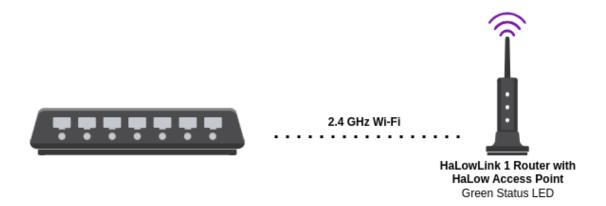
If it's not possible to connect your HaLowLink via Ethernet, you can connect your HaLowLink via 2.4 GHz Wi-Fi. You should only do this if Ethernet is not possible, as it will require your HaLowLink to act as a router, forwarding traffic from 192.168.12.x over the Wi-Fi link.
