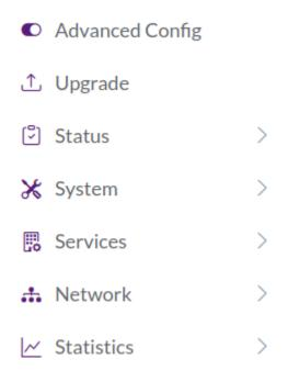
This will allow you to view detailed information about your device, change low-level configuration, install additional software if you have an internet connection (via **System** -> **Software**), and even access the Linux terminal (via **Services** -> **Terminal**).
