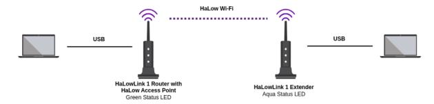
If you're currently just experimenting with HaLow's amazing range and penetration, the easiest way to test this out with a HaLowLink 1 is to have two devices and two laptops, where the laptops provide power to the HaLowLink. This allows you to easily move around.
