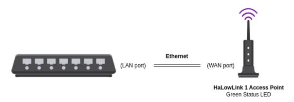
The primary use case for a HaLowLink 1 is to add HaLow support to your existing network, allowing any HaLow-enabled client to work in the same way as any other Wi-Fi client.
