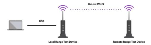
The Range Test application is designed as a simple way to analyse HaLow network performance by automating iPerf3 tests and collecting real-time statistics. It is a useful tool for quickly assessing signal strength, data throughput, and connection quality across different environments.
