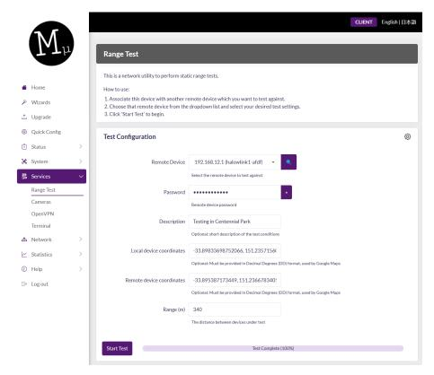
Before using this application ensure that all devices under test are running the same version of Morse OpenWrt. This tool can run with different types of evaluation kit (i.e. between an HaLowLink 1 and an EKHO1) but the software versions must be the same. To use the range testing tool:
