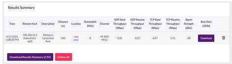
This result can be deleted by clicking the trash icon, or a JSON file containing all the raw data can be downloaded via the 'Download' button, which is intended to help engineers with remote debugging. The 'Download Results Summary (CSV)' button yields a CSV file of all the data represented in the results summary.
