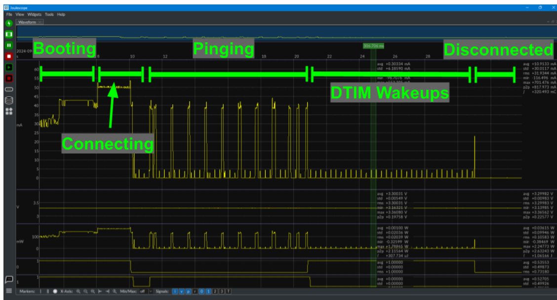
Figure 64. Example current consumption profile from ping application.
