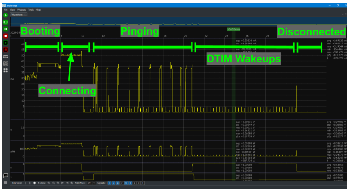
Figure 63. Example current consumption profile from ping application.
